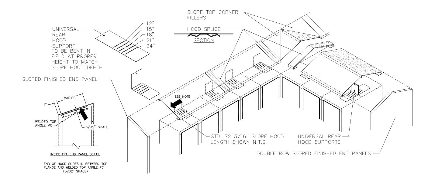
SLOPED FINISHED END PANEL & HOOD DETAIL
