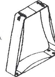
Recommended pedestal locations apply to all pedestal types except as noted. For pedestal spacing on custom benches, contact engineering for guidance. Hardware for attachment to benches is included with pedestals. Pilot holes must be drilled by the installer/end-user. Use appropriate hardware (not included) for anchoring pedestals to the floor.
